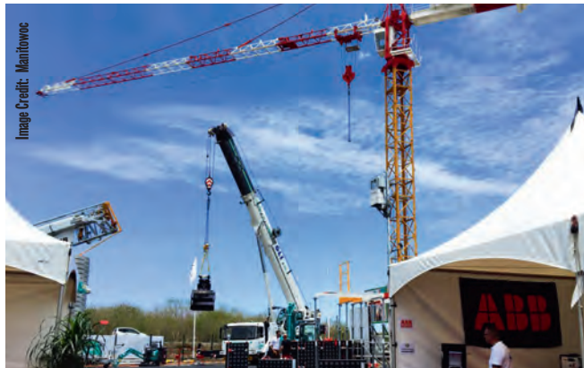
A Grove GMK4100L-1 all-terrain crane and Potain Hup 40-30 self-erecting crane was displayed at Le Port.
